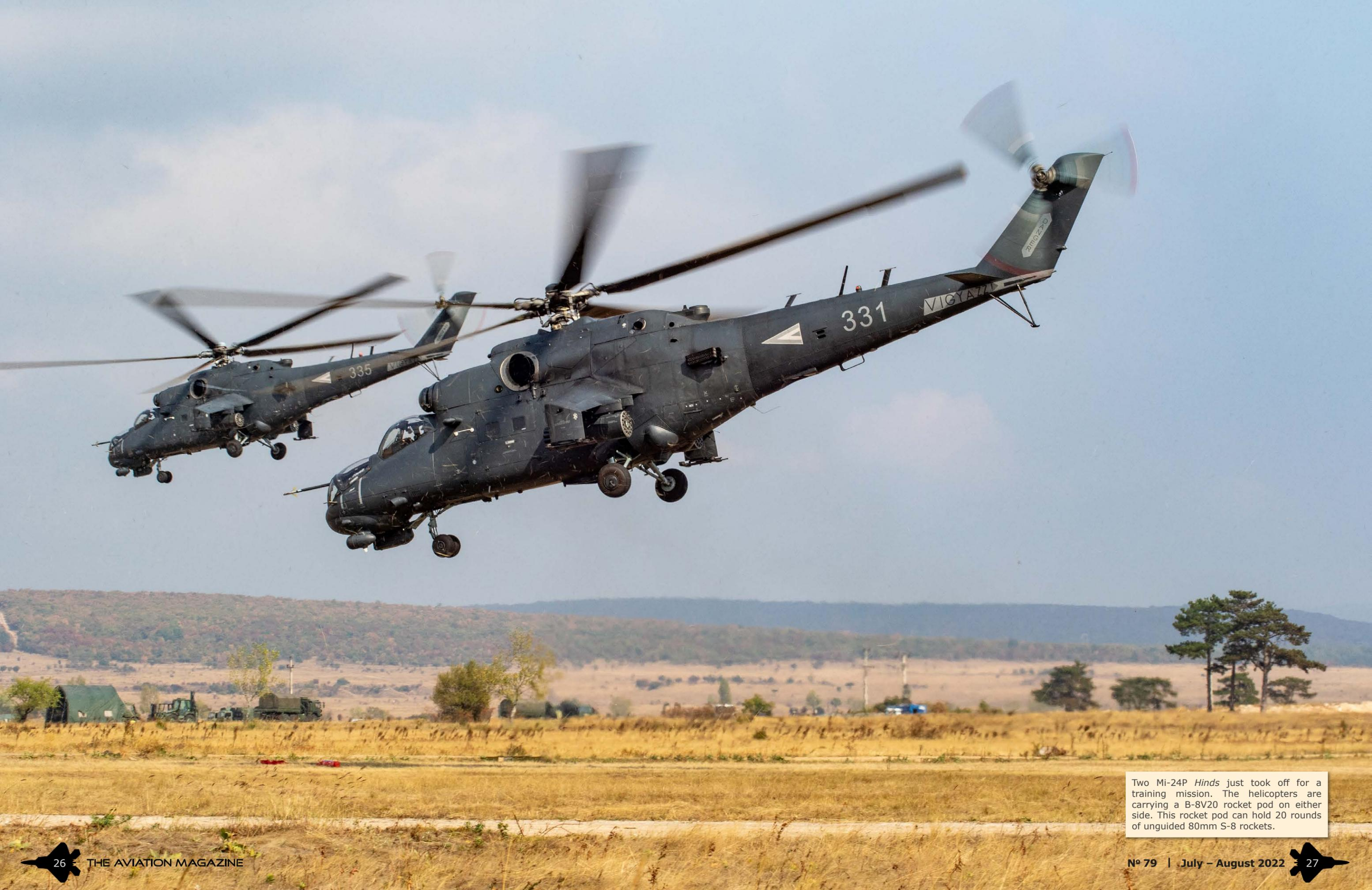
Two Mi-24P *Hinds* just took off for a training mission. The helicopters are carrying a B-8V20 rocket pod on either side. This rocket pod can hold 20 rounds of unguided 80mm S-8 rockets.
