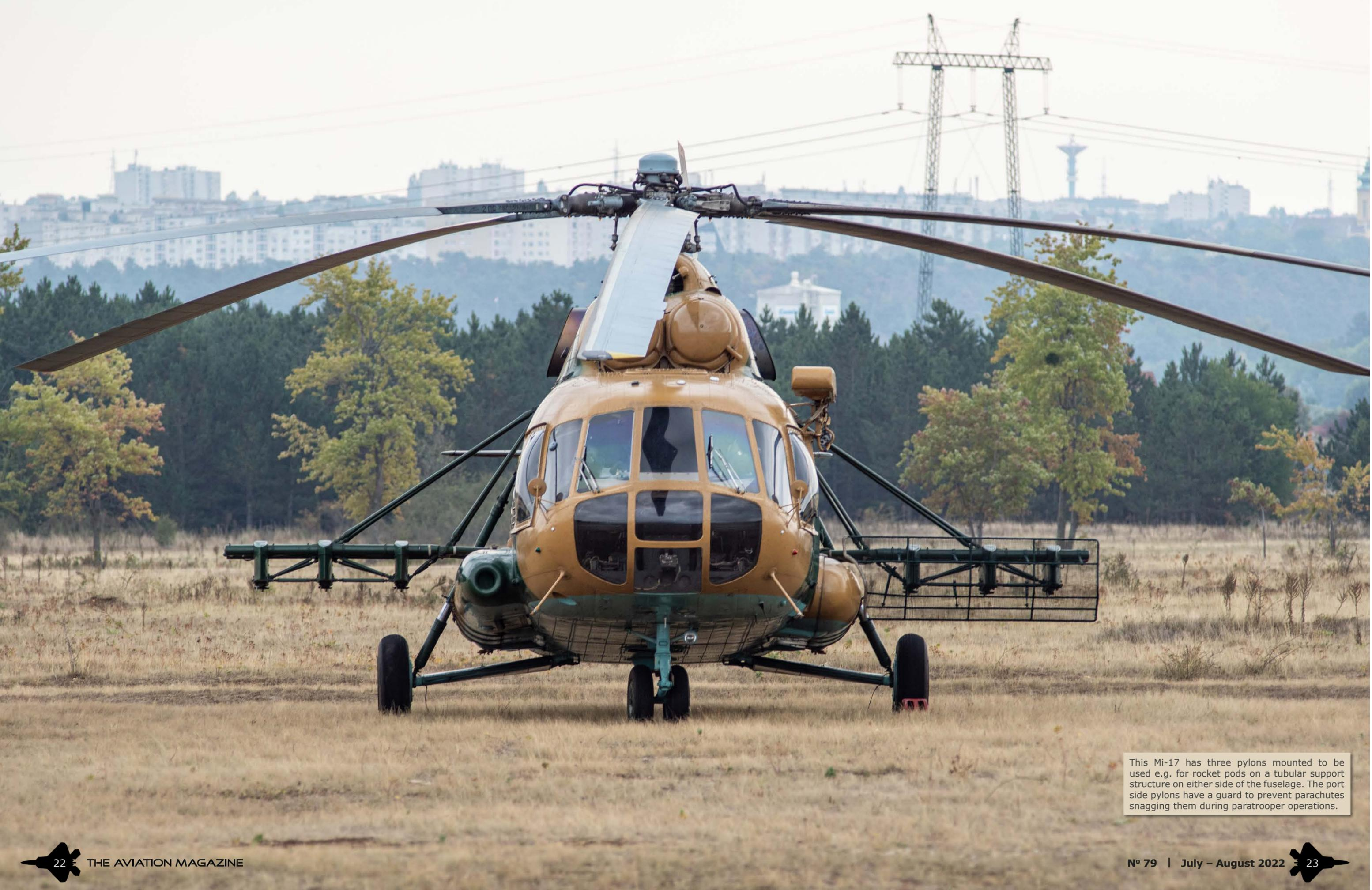
This Mi-17 has three pylons mounted to be used e.g. for rocket pods on a tubular support structure on either side of the fuselage. The port side pylons have a guard to prevent parachutes snagging them during paratrooper operations.
