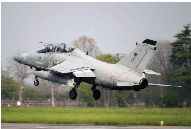
Capability Upgrade) was launched for 55 AMXs (43 single-seat AMX and 12 double-seat AMX-T) of the Italian Air Force adding a new multi-function colour cockpit display, laser INS, Night Vision Goggle (NVG) capability and the aircraft was able to drop Joint Direct Attack Munition guided bombs. In 2012 the Italian military designation for the AMX was A-11A and for the AMX-T it was TA-11A. After the ACOL upgrade programme the Italian military
