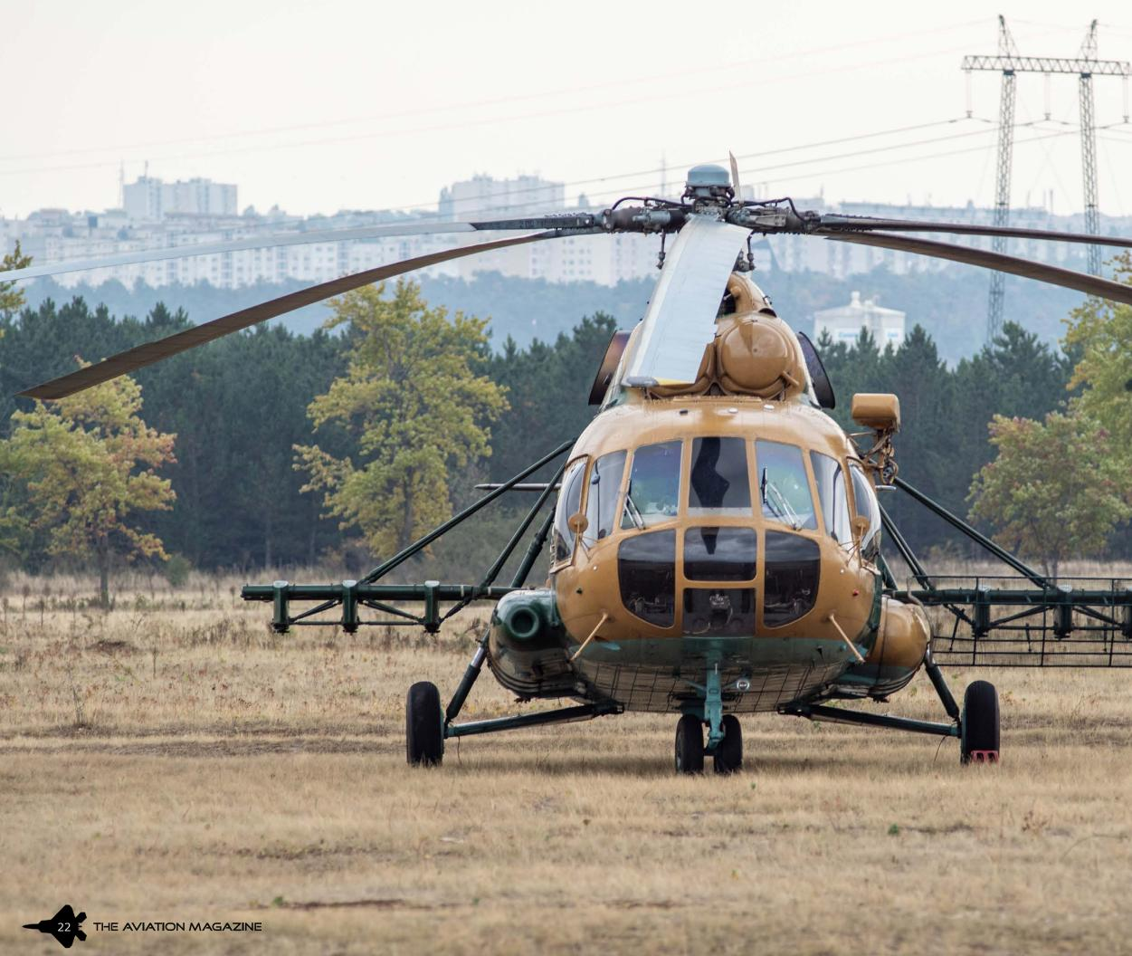
This Mi-17 has three pylons mounted to be used e.g. for rocket pods on a tubular support structure on either side of the fuselage. The port side pylons have a guard to prevent parachutes snagging them during paratrooper operations.
