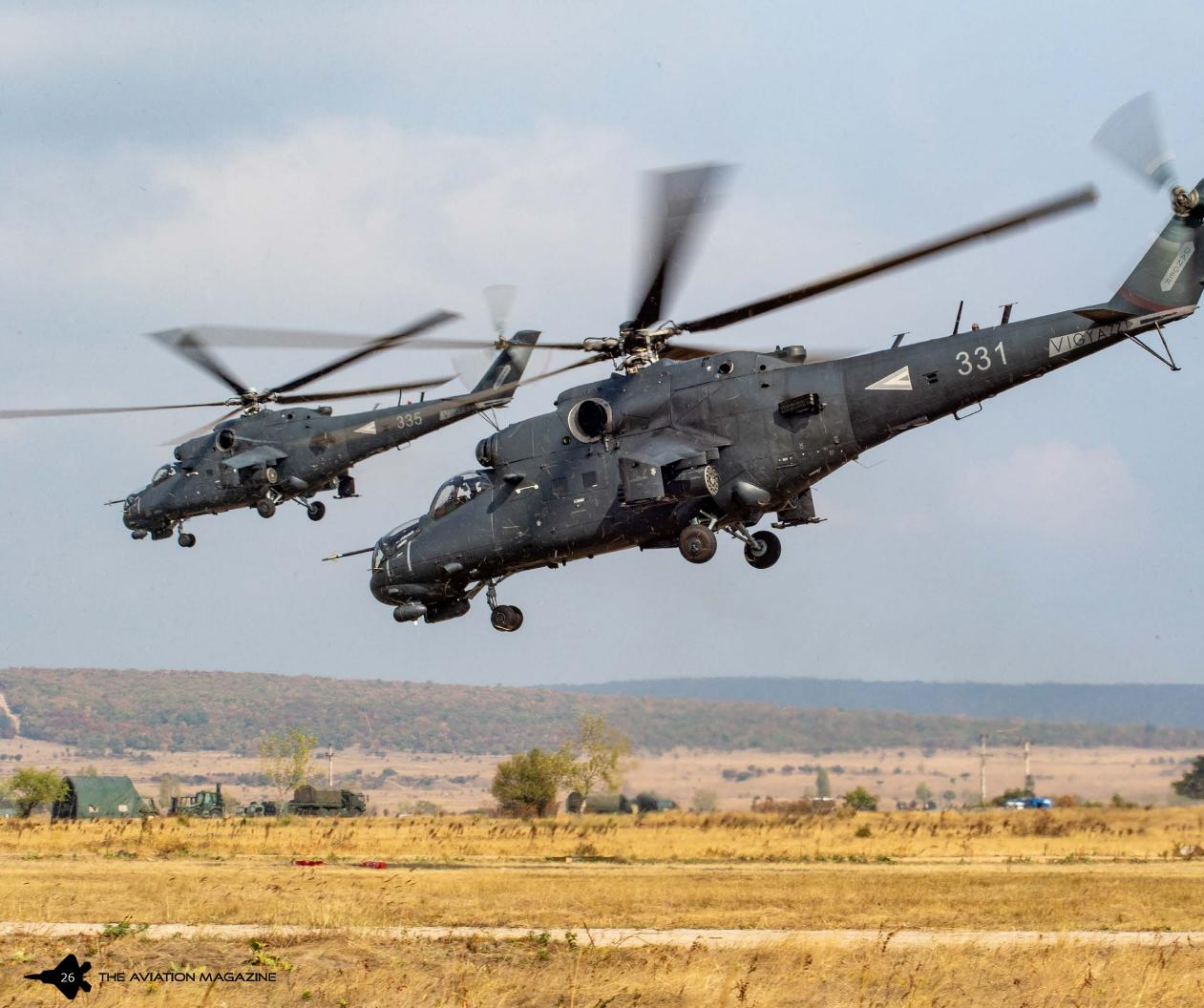
Two Mi-24P *Hinds* just took off for a training mission. The helicopters are carrying a B-8V20 rocket pod on either side. This rocket pod can hold 20 rounds of unguided 80mm S-8 rockets.
